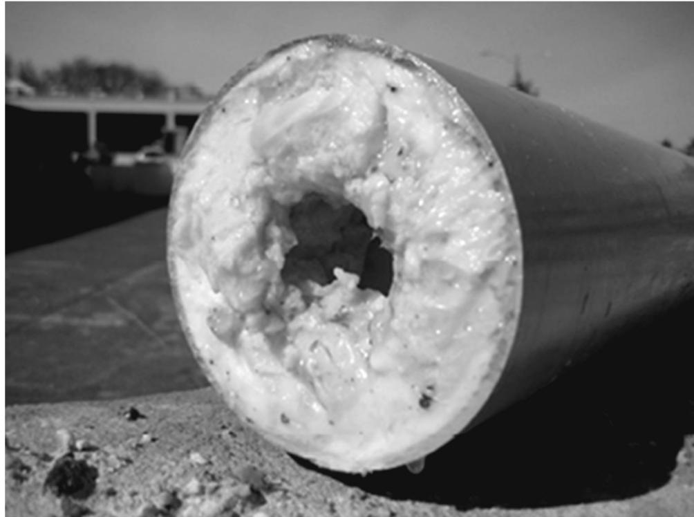
This is what a sewer pipe clogged with kitchen fats, oil, and grease looks like (see picture). When cooking oil is poured down the drain, it gels and solidifies inside of pipes, sewage lines, and sewage lift stations. This constricts water flow, causing back ups and equipment malfunction, which ultimately lead to sewage spills and overflows from Hillsborough County's wastewater collection system.
